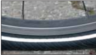
That’s how it shouldn't look. The inflation pressure is far too low here.
