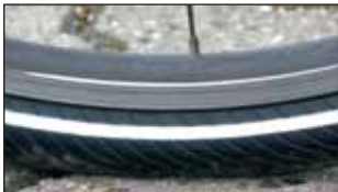
That’s how it should look. The tire is hardly deformed under the weight of the rider.
