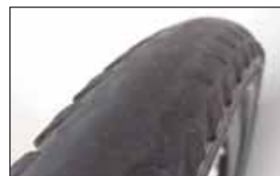
Tread is worn out. Rubber is still present. This tire can still be ridden.
