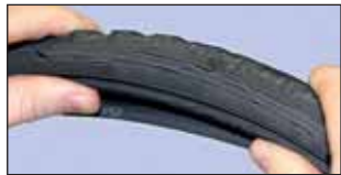
Fatigue Cracks
