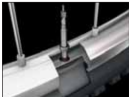
Too large inner valve hole
